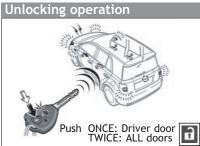
**NOTE:** If a door is not opened within 30 seconds of unlocking, all doors will relock for safety.
